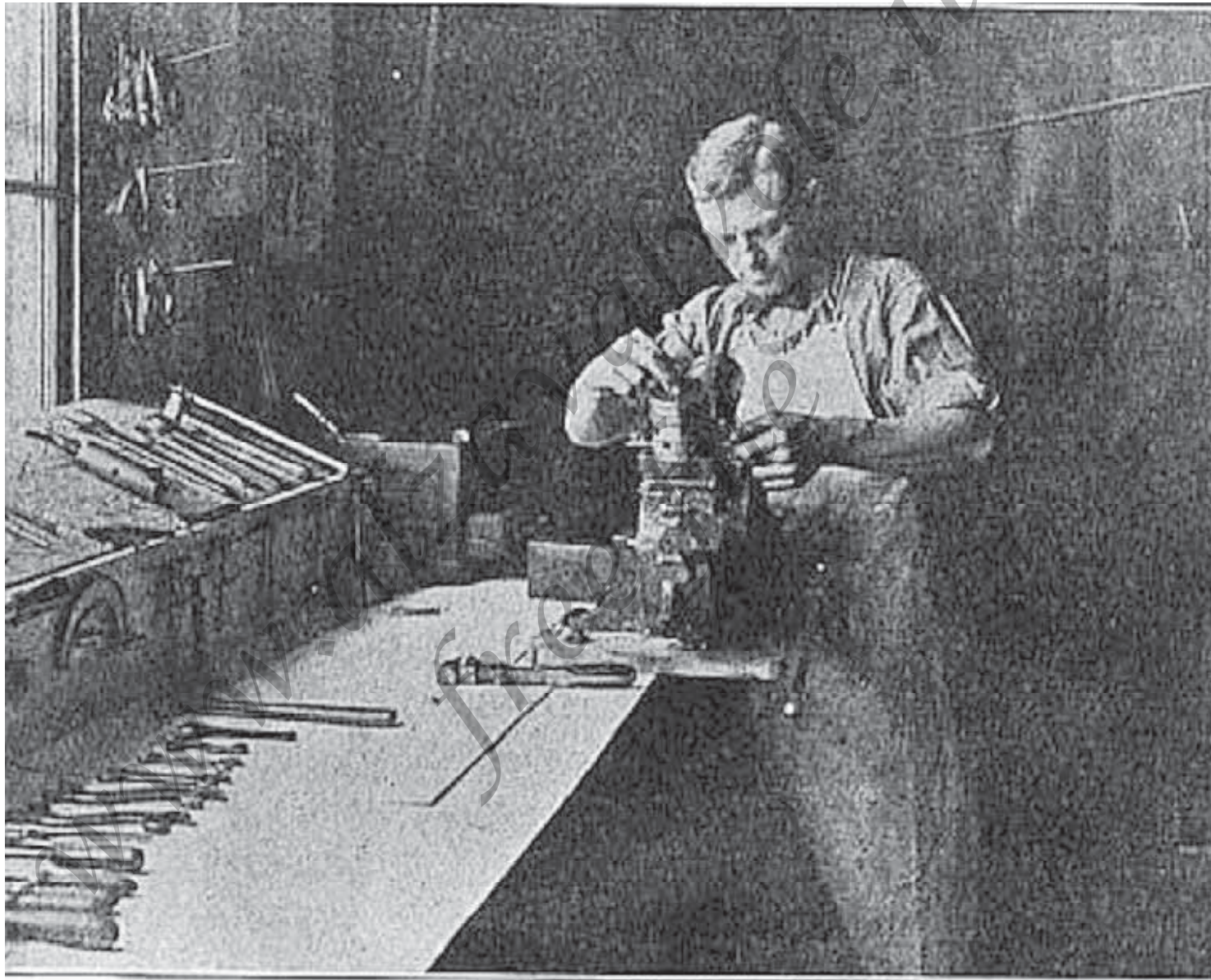
Fig. 369.—How to Test Pistons for Correct Alignment.
